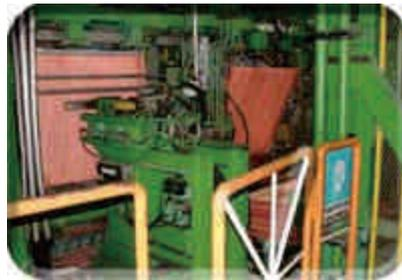
3. Copper plates are washed and stripped off at CWSM (Cathode Washing & Stripping Machine)
