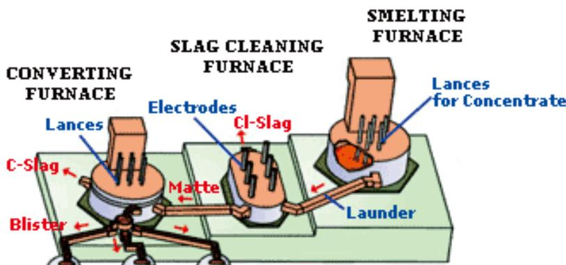
covered launders, through which all the molten materials are continuously transferred by gravity.
