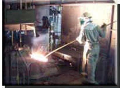
Matte and flux (limestone) are reacted with oxygen-enriched air to form blister copper and then separated from the slag by difference of specific gravity. Slag (Cu14%) is returned to S-furnace, and blister copper is siphoned out and forwarded to Anode furnaces.
