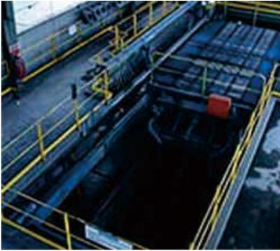
In the final process, concentrate from the barn is loaded onto vessels on conveyors. Loading onto a concentrate vessel is partly conducted at the concentrate jetty and the vessel is then moored to the (offshore) Sea Buoy A to complete the loading process using barges. The use of barges is necessary because the water depth does not allow full loading onto the vessel. We ship our concentrate aboard more than 100 vessels every year.
